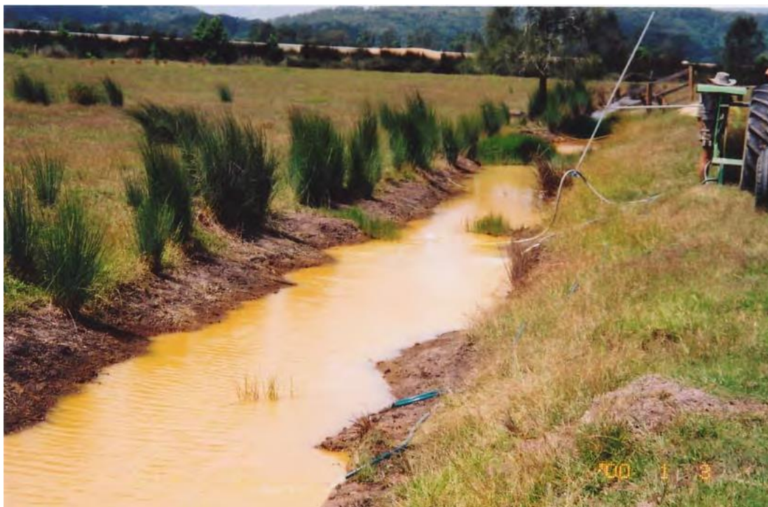
Figure 7-10 In-stream dosing system immediately after \text{CaCO}_3 was added and dissolved metals (in particular iron) precipitated (Green, 2005)
