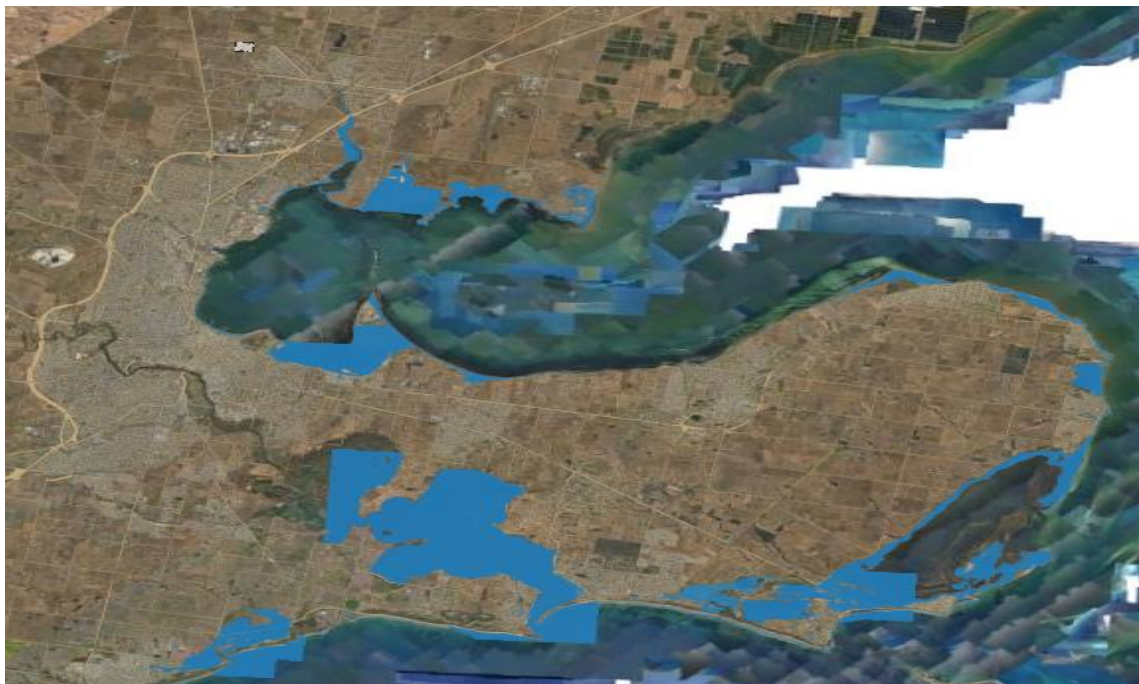
Coastal areas around the City of Greater Geelong and Bellarine Peninsula showing modelled flood extents for the 1% AEP event + 0.8m sea level rise (Photo credit: Corangamite CMA GIS flood mapping)
