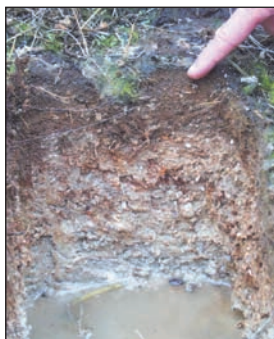
Fig. 1: Once disturbed and exposed to oxygen in the air, acid sulfate soils go on producing high concentration sulfuric acid.
